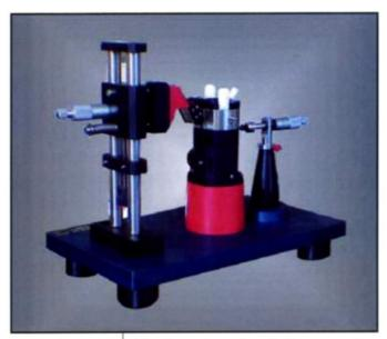
The Long term incubation muscle research system is primarily designed for studies where the effect of a mechanical, biological or other intervention is monitored over time. Its primary use is intact living muscle preparations. It combines the versatility of the rugged and stable force transducer of the KG series with fast and sensitive force measurements.
