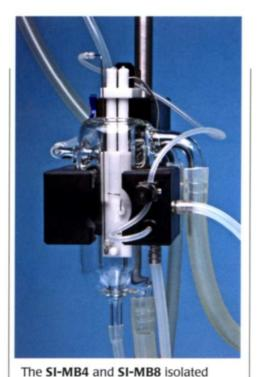
The SI-MB4 vertical tissue bath is shown with all four channels (below). The closeup (right) shows a single tissue bath with a tissue holder mounted in the bath.
