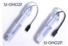
All three tissue holders are designed for simple and accurate preparation mounting. As the tissue holder slides into the tissue bath, its size significantly lowers the volume of liquid in the tissue bath.
