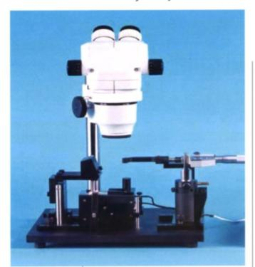
Combining the versatility of the KG force transducers and a solid platform for mechanical studies, the Muscle Tester (Basic Research System) can be equipped with a linear motor and laser diode for running advanced muscle studies.
